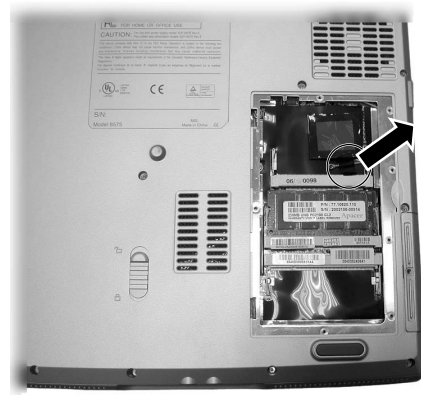
Figure 2-15 Remove the tape from the antenna
