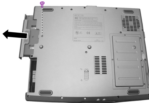
Figure 2-12 Remove one screw to loose the CD/DVD-ROM drive
