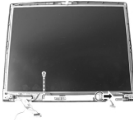
Figure 2-20 Remove the inverter board
