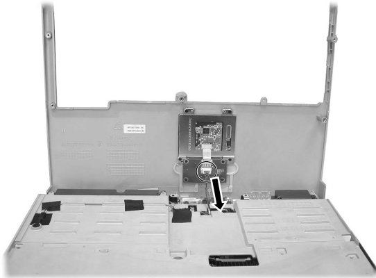
Figure 2-23 Remove the base unit cover
