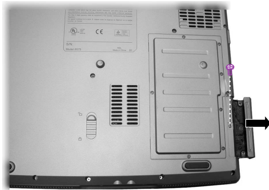
Figure 2-10 Remove HDD module
