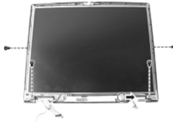
Figure 2-19 Remove LCD panel
