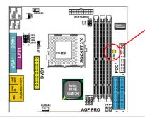
NOTICE : When LED1 light is on , meaning that 3.3V is conducting DIMM slots , please do not add or remove memory modules .
