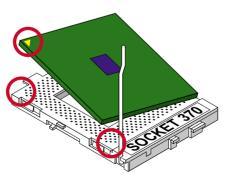
3. Make sure that the CPU positions in the socket tightly, and then put the lever down to complete the CPU installation.
